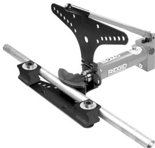
Figure 10 – Loading the Pipe
