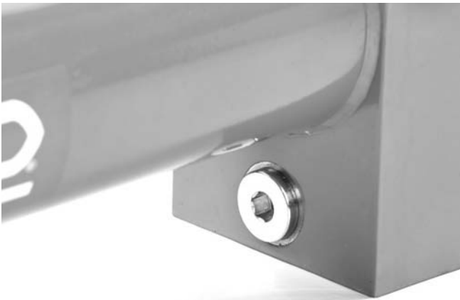
Figure 19 – Hydraulic Oil Drain Plug and Access to Filter
